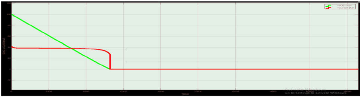
Figure 1.64:- SOC & CURRENT WAVEFORM OF DISCHARGE OF PARALLEL CONNECTED LITHIUM ION-LITHIUM ION BATTERY WITH LOAD AS STEP SIGNAL FOR 6 HOURS
