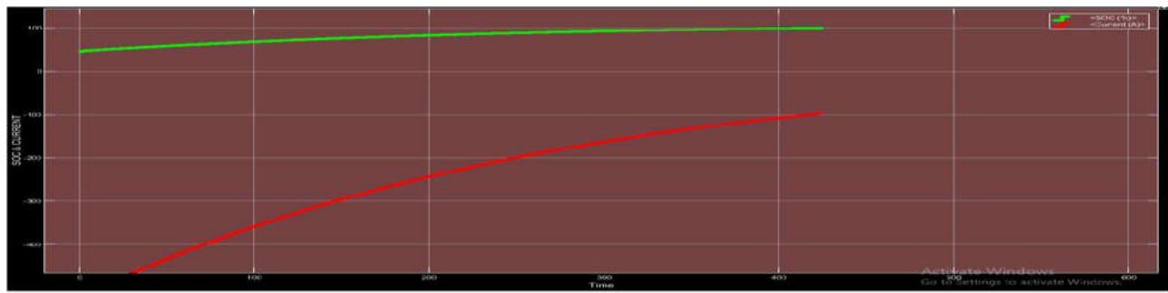
Figure 1.2:- SOC & CURRENT WAVEFORM OF LEAD ACID BATTERY CHARGING FOR 425 SECONDS
