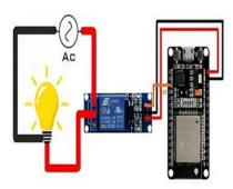
Fig. 5: Circuit Diagram of IOT Model
