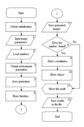
Fig. 1: Elementary Flow Chart of Augmented Reality
