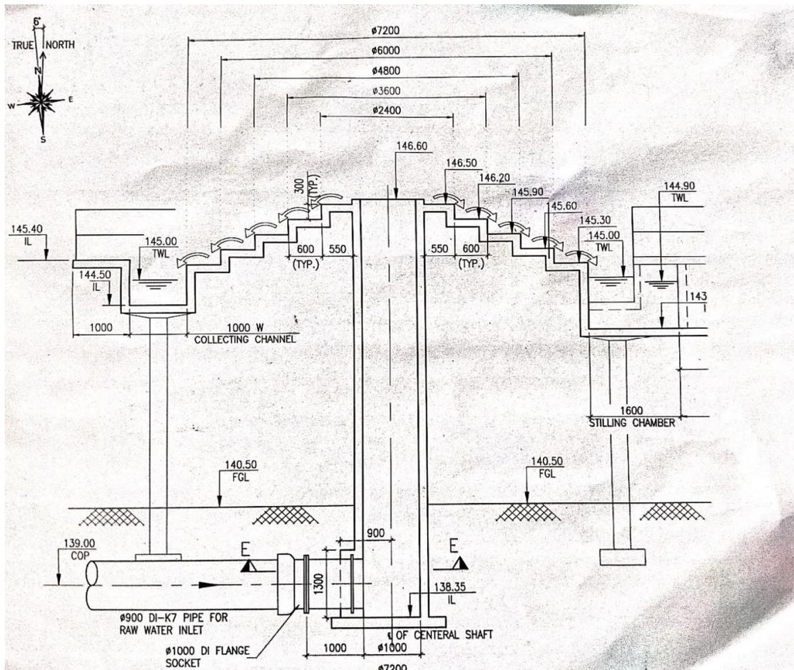
Fig-1 showing typical cross sectional view of cascade aerator.
