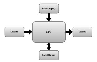
**CPU :-** The Central Processing Unit (CPU) is the brain of the device. It analyzes the data that the camera records. The block diagram shows a Raspberry Pi which is a minicomputer that can be used for various purposes including image processing.
